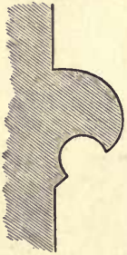
Impost of North Transept Arch.
